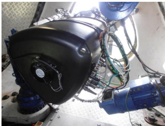
Photo of nacelle-based lidar installed in the spinner of a wind turbine.
